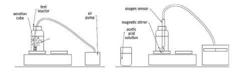
Figure 2. Scheme of the research stand for conducting the OUR tests.
