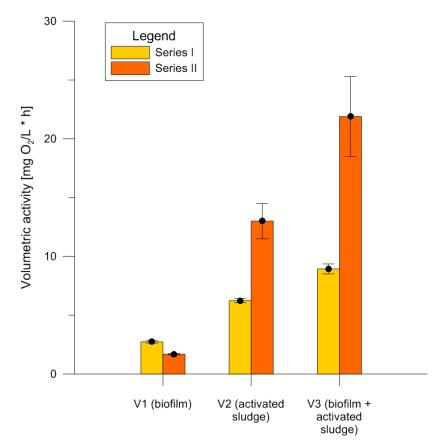
Figure 4. Comparison of volumetric activity of microorganisms developed as biofilm and activated sludge.
