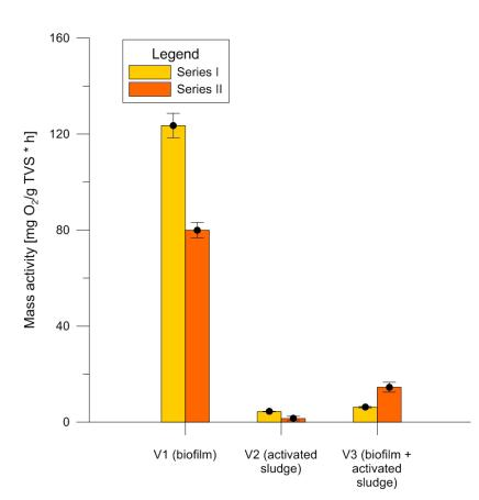
Figure 5. Comparison of mass activity of microorganisms developed as biofilm and activated sludge.
